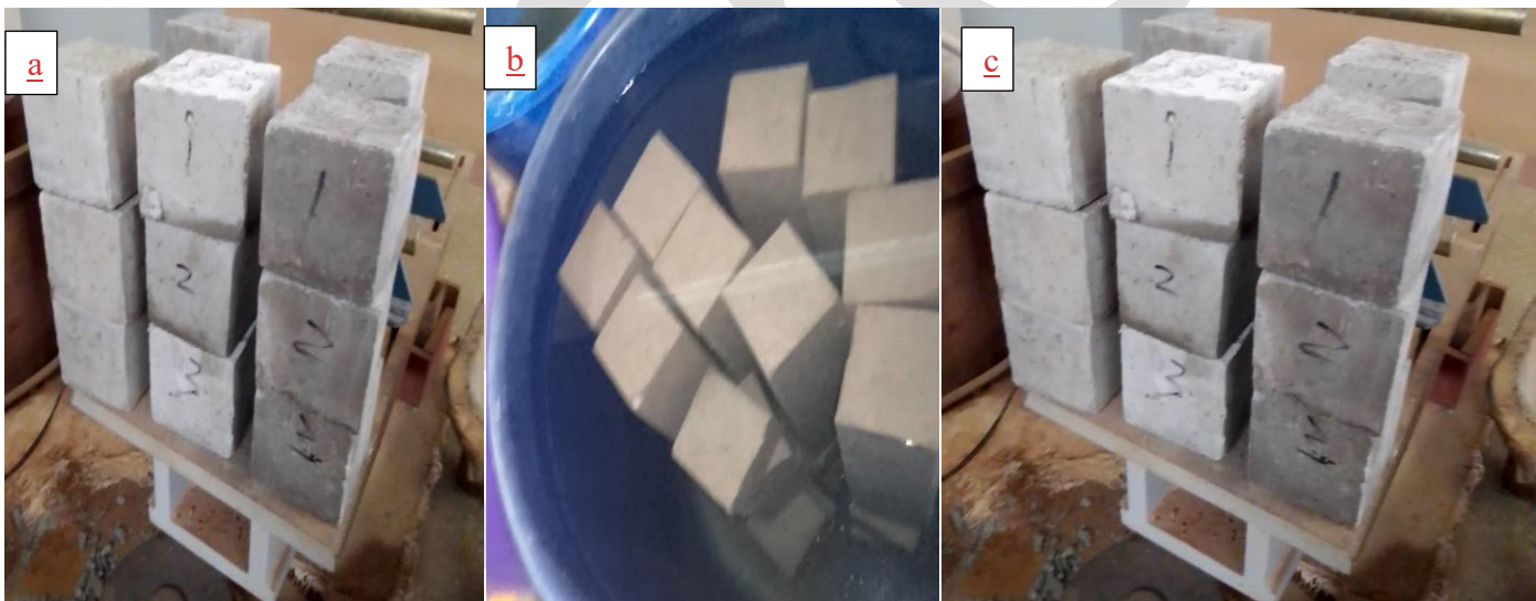
Figure 3: Concrete cubes: (a) initial setting, (b) curing, (c) ready for testing
