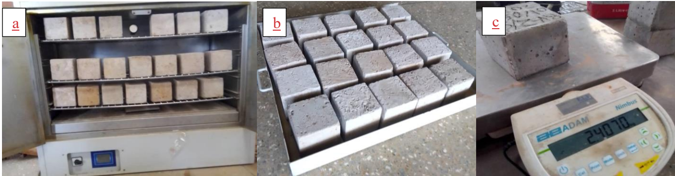
Figure 4: Water absorption test: (a) oven-drying of specimens, (b) air-drying of specimens after oven-drying, (c) weighing of specimen
